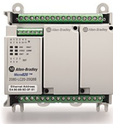
Figure 1: The unitary Micro820 PLC from Allen-Bradley
