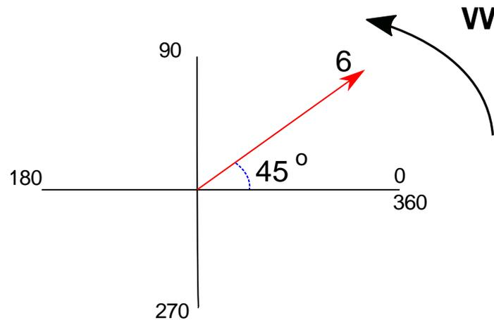
The phasor featured above represents a sine wave with a peak value of 6 (perhaps volts) and an angle of 45 degrees. Here we adopt the convention that the peak value of the sinusoid is used as the phasor length.
