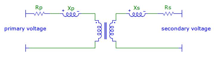
Figure 2 Basic transformer equivalent circuit
