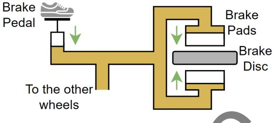
Fig.2.3: A schematic of a vehicle's braking system
