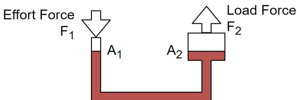
Fig.2.2: Hydraulic diagram
