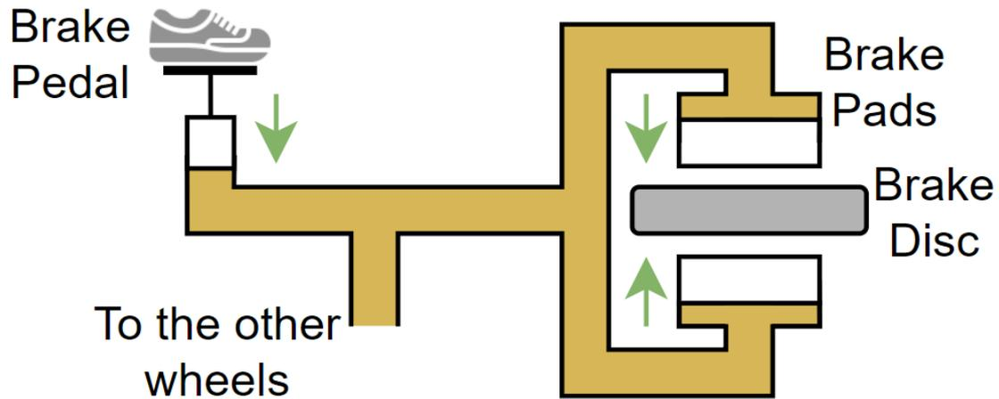
Fig.2.3: A schematic of a vehicle's braking system
