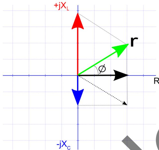
The black arrow represents resistance. The current through a resistor is always in phase with the voltage across it. We place resistance on the horizontal axis.
