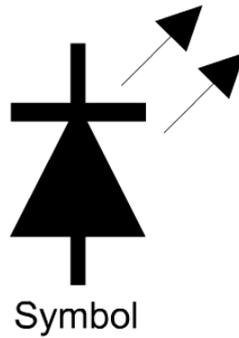
When electrons jump across the junction between the n-type and p-type material to combine with a hole, their energy level changes. In a silicon diode, this energy is converted to heat, but some materials, such as Gallium Arsenide (GaAs), will convert this energy to heat and also to light. Depending on the material used, LEDs that emit red, green, yellow and blue light can be manufactured.
