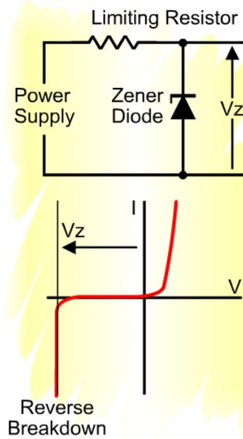
Unlike a standard diode, a zener diode is operated in reverse breakdown mode, with current flowing from cathode to anode.
