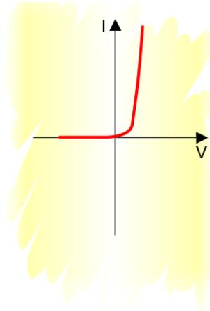
When forward biased, the diode will conduct well and allow a current to pass. When reverse biased, the diode does not conduct and will stop current flowing.
