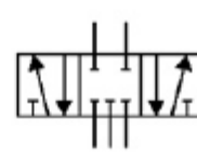
5 port, 3 position DCV all ports blocked in center
